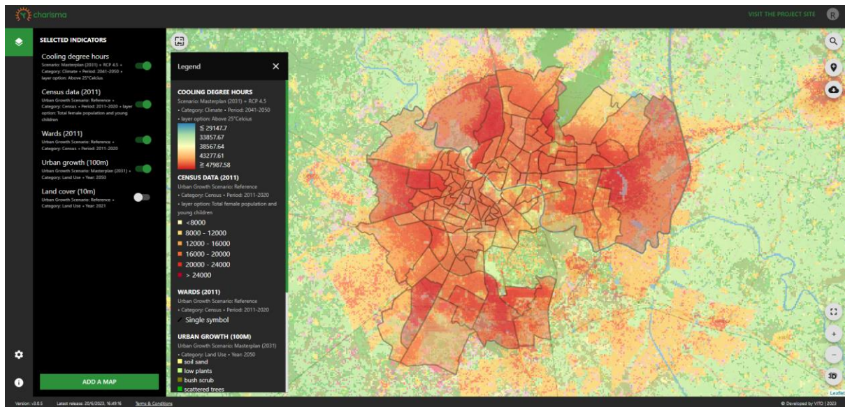
Figure 36: By overlaying multiple layers (“COOLING DEGREE HOURS”, “CENSUS (2011)”, “URBAN GROWTH (100M)”) areas within the city which require interactions in terms of cooling requirement, become evident.
