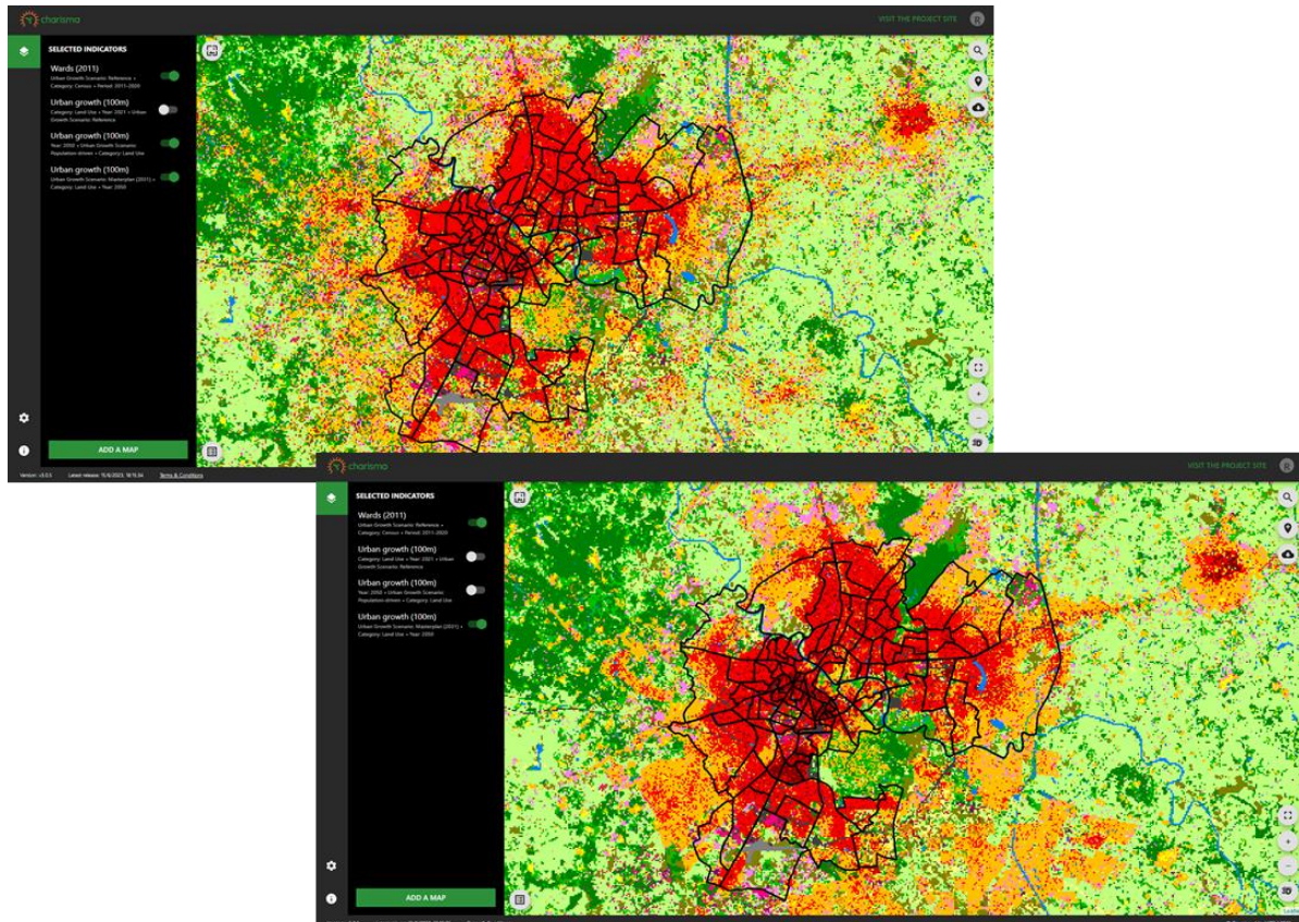
Figure 23: Masterplan assessment. (Left) Simulated urban extent in 2050 if population-driven, without intervention. (Right) Urban growth with the 2031 Masterplan in place.
